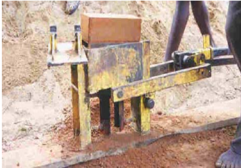
Figure 3 Stabilized soil block manufacturing in Africa(DTU, 2000b)
